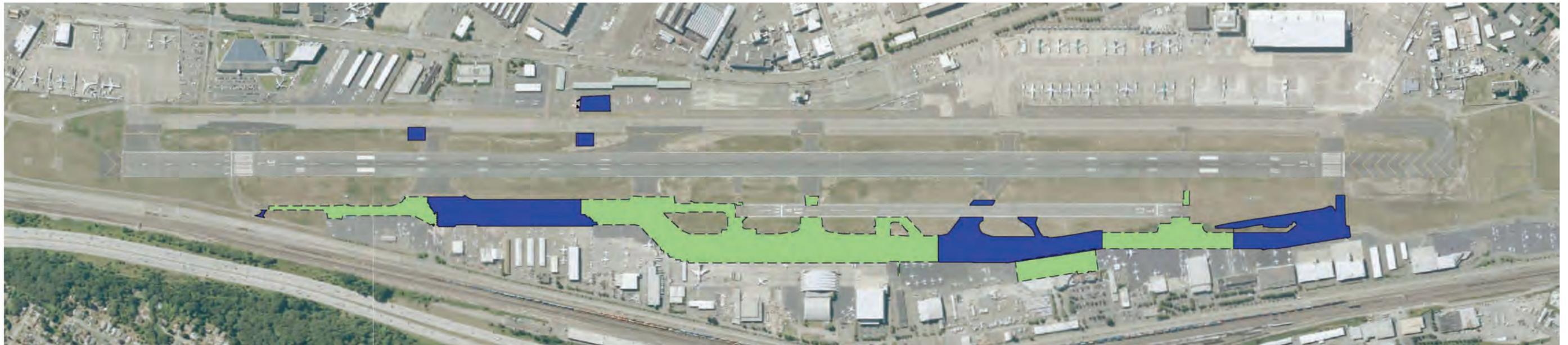
This graphic shows the overall limits of the work that will be undertaken as part of the Taxiway Alpha Rehabilitation Project. Blue areas indicate work that is in Package No. 1. Green Areas indicate work that is in Package No. 2.
